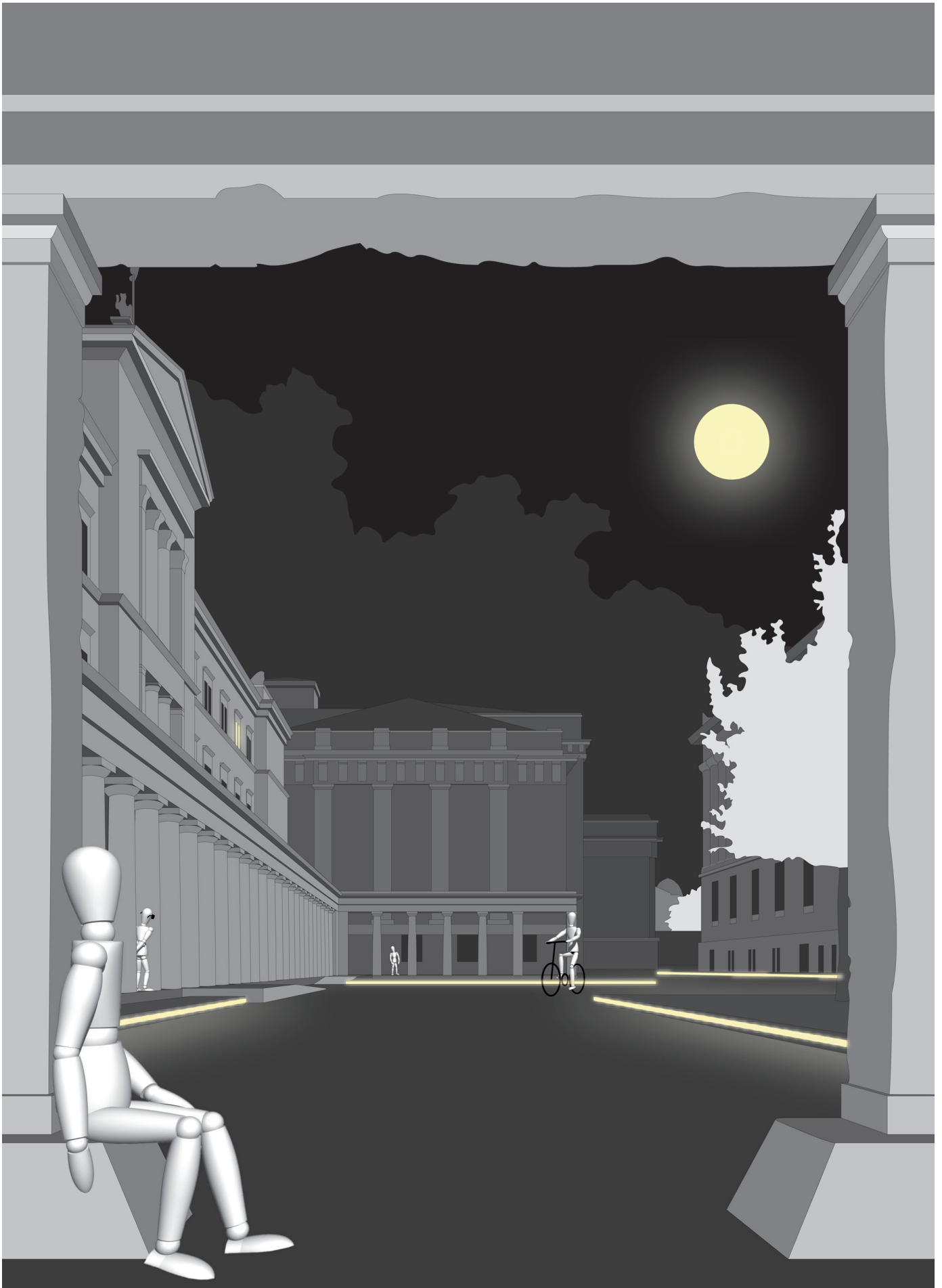
Even lighting of the pathways to support orientation. Illustration based on: Kolonnadenhof Old National Gallery and New Museum
